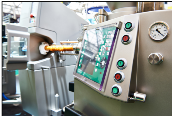
Sausage casing “clipping” machine.
